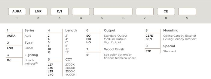
1. Interior mounting must be in a location without affect from winds. 2. Lumen output based upon 3000K CCT.
