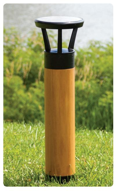
**OPTICAL SYSTEM**: Uses high-output LEDs with a 100,000 hour L70 life. Typical solar lumen output is 239-370 lumens and AC powered output of 740 lumens (Type III) and 1200 lumens (Type V). Available with warm white (3000K), neutral white (4000K), and amber (595nm) color temperatures.
