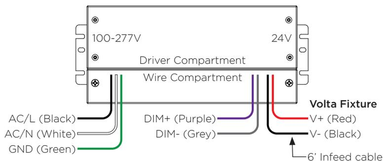
Suitable for indoor or outdoor use. Horizontal or vertical mounting. End and side knockout locations of 7/8" (1/2" trade size"). When installing multiple power supplies, separate the enclosures by at least 3" of space from edge to edge to prevent a rise of ambient temperature between the power supplies.
