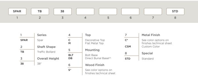
1. Direct burial designed to be embedded in soil. Embeddment into concrete can cause corrosion with aluminum base.
