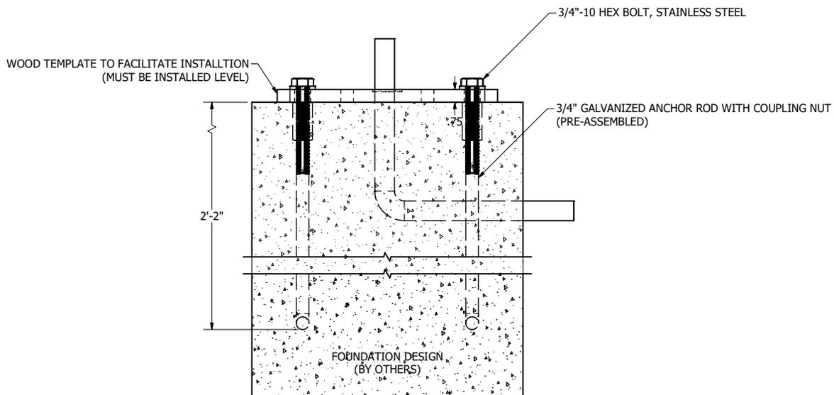
Assemble anchor bolts to template as shown above.
