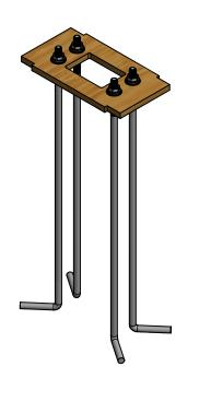
Use baseplate template to install anchor bolts. Slope concrete away from baseplate. After concrete has set, remove base accent panels from bollard and set aside. Remove template and set bollard on top of anchor bolts. Tighten flange nuts until bollard is secure. Reattached accent panels.
