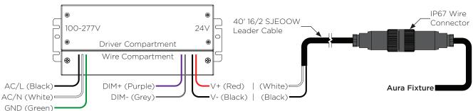
Suitable for indoor or outdoor use. Horizontal or vertical mounting. End and side knockout locations of 7/8" (1/2" trade size"). When installing multiple power supplies, separate the enclosures by at least 3" of space from edge to edge to prevent a rise of ambient temperature between the power supplies.
